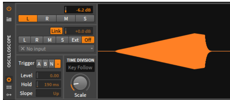
Figura 58. Prueba envolvente de amplitud - Attack: 1000ms; Decay: 50ms, Sustain: 0.8; Release: 50ms.
