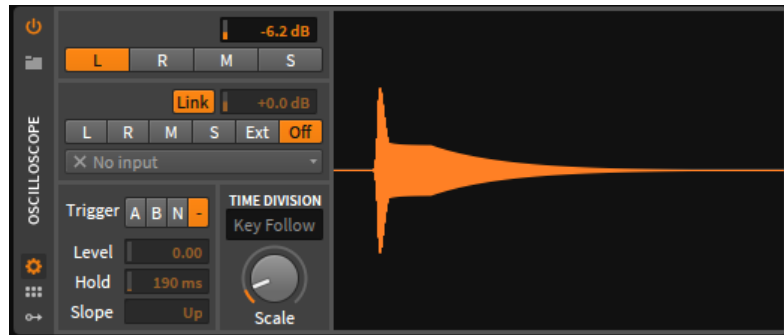
Figura 59. Prueba envolvente de amplitud - Attack: 50ms; Decay: 50ms, Sustain: 0.3; Release: 1000ms.
