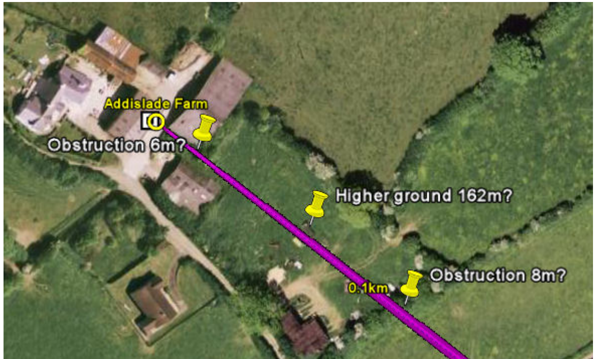
Figure 3.50: Obstructions and higher ground near Addislade
