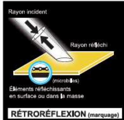
Figura 3-3 Retroreflexion. (Frédéric Boily, 2014).
