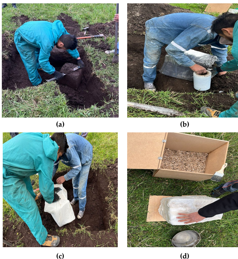
Figure 2. Soil block extraction. (a) Soil block sampling, (b) conservation of extracted blocks, (c) block preparation, and (d) sample before transport.
