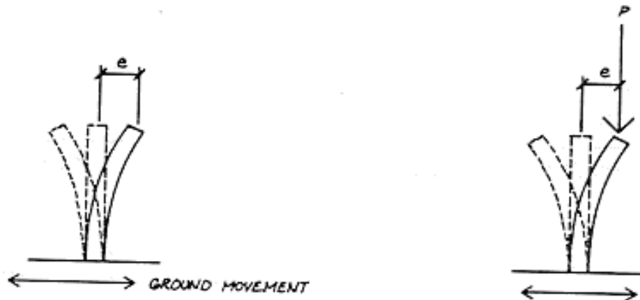
Figure 11: The P-e effect. The stresses caused by the P-e moment occur concurrently with the other stresses induced by the earthquake and gravity. At a particular instant, the stresses may all be additive.
