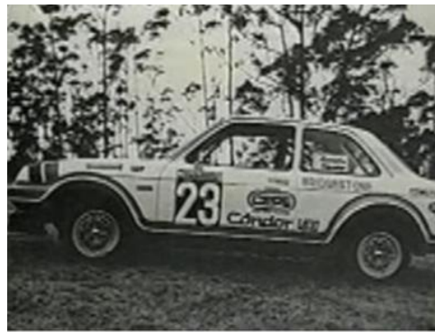
CONDOR: Fiber Glass bodywork . The first vehicle under Ecuatorian Brand - 1978
